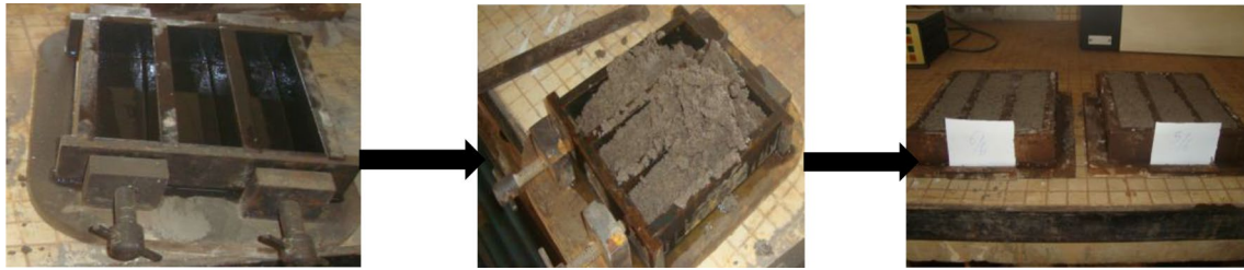
Fig. 3 Prismatic Mould. Mould filling. Mould leveled and labeled
