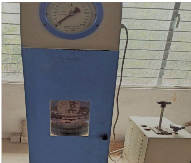
Fig. 3 Setup of Split Tensile Strength Test
