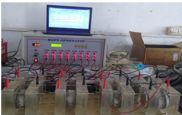
Fig. 4 RCPT test setup to test the GC samples
