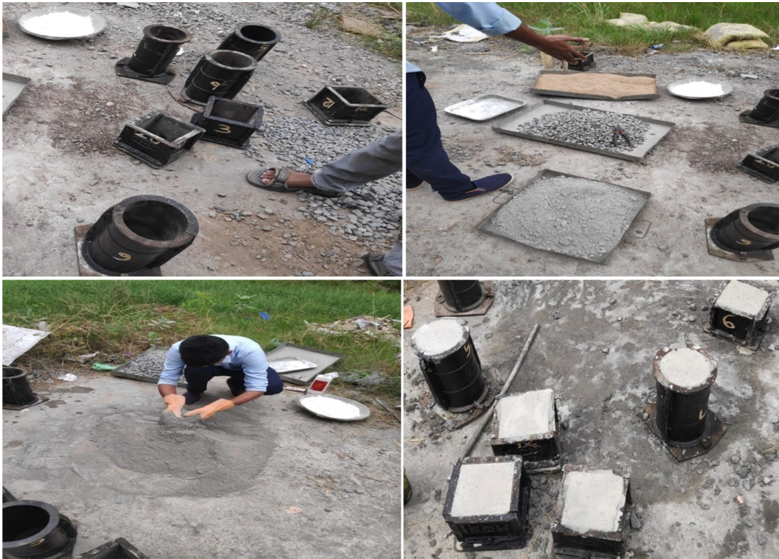
Fig. 9 Placing of concrete in the various specimen
