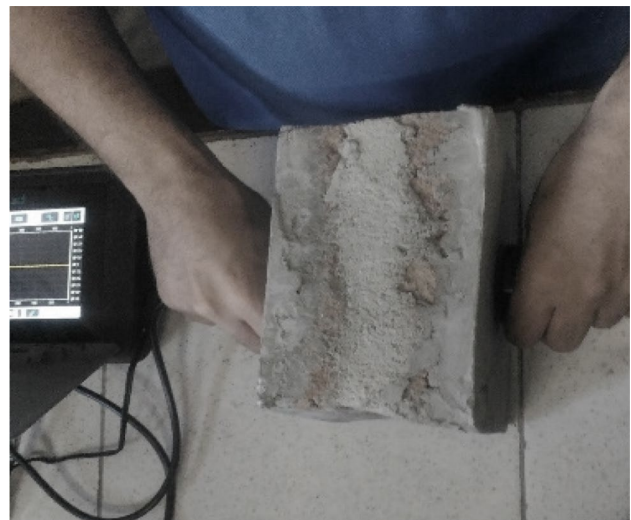
Fig. 4 UPV measurements in a sample
