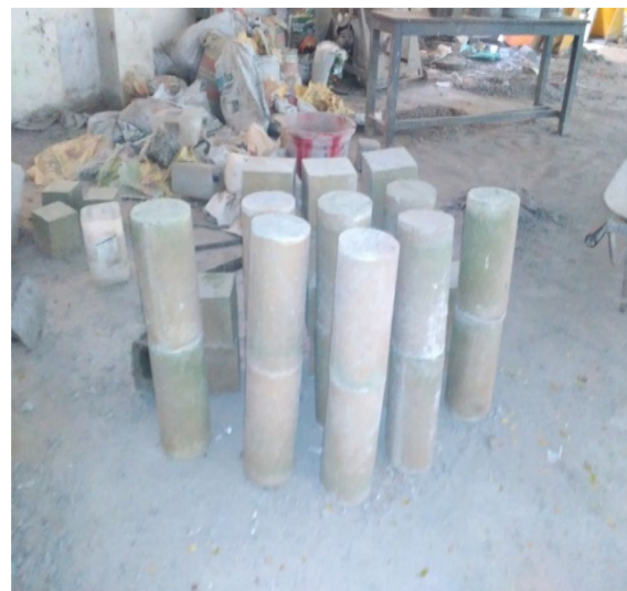
Fig. 4 Specimens for testing after curing
