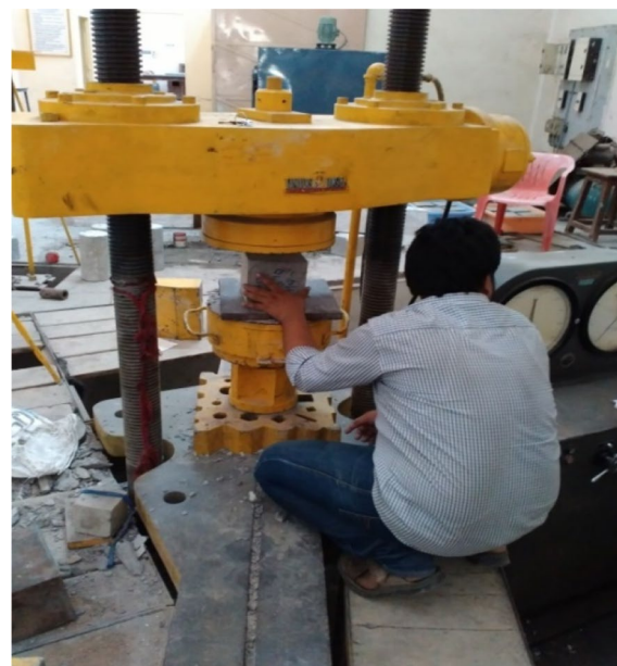
Fig. 5 Testing of specimen under compression
