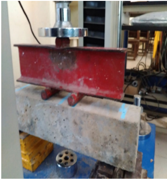
Fig. 6 Testing of the specimen under flexure
