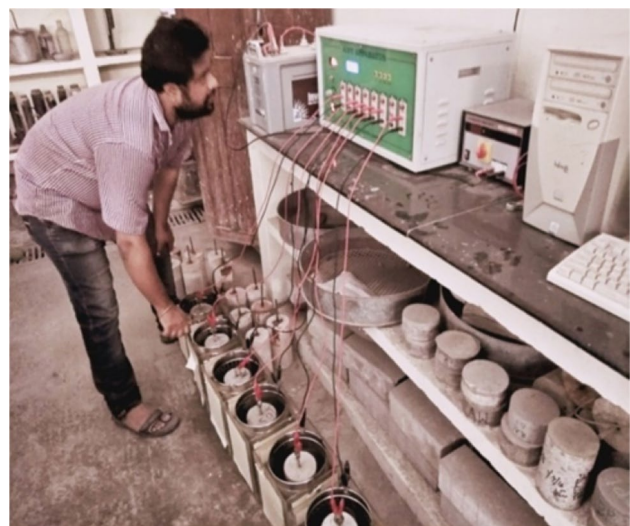
Fig. 15 Test setup for ACPT
