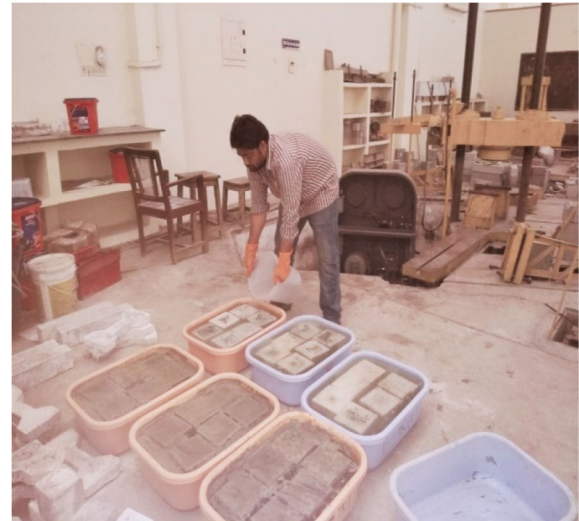
Fig. 8 Pouring of acid in the tubs
