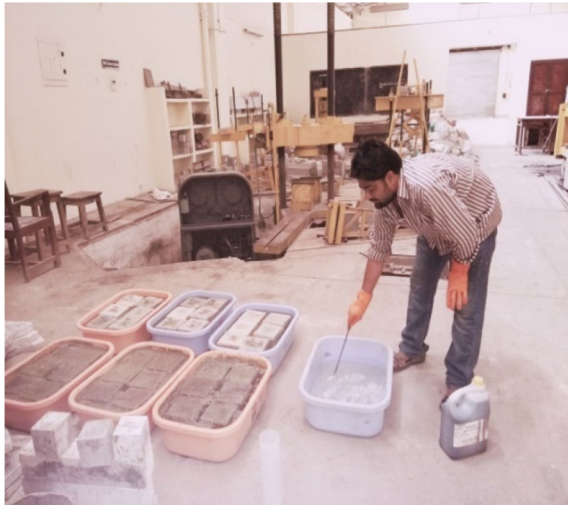
Fig. 7 Preparation of acid to study acid attack
