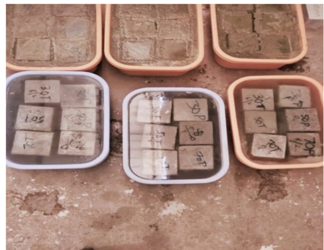
Fig. 9 Concrete specimens in acid
