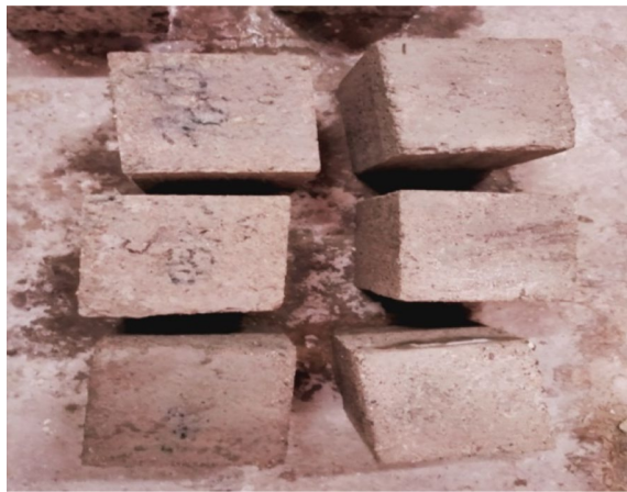
Fig. 10 Concrete specimens after 56 days in acid
