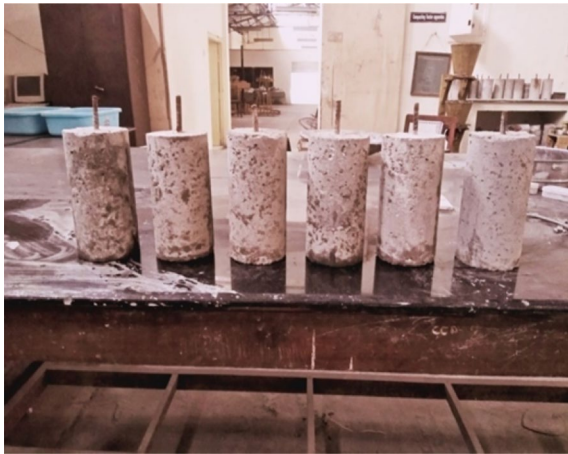
Fig. 16 Concrete specimens after the test
