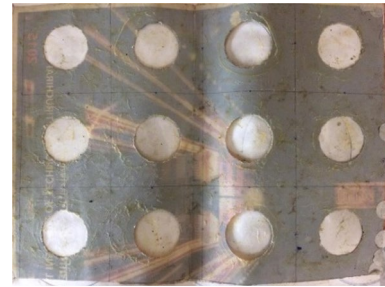
Fig. 6 Grid sheet of 10 × 10 cm size for UPV testing
