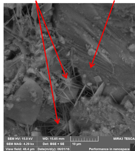
Fig. 16 Electron microscopy scanning obtained for contaminated series of mortars at 28 days (submerged healing condition)
