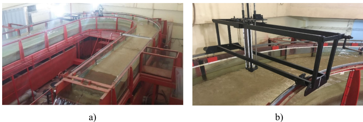
Fig. 1 a Laboratory channel used in the experiments, b The device collecting the temporal variation of the scour hole depth
