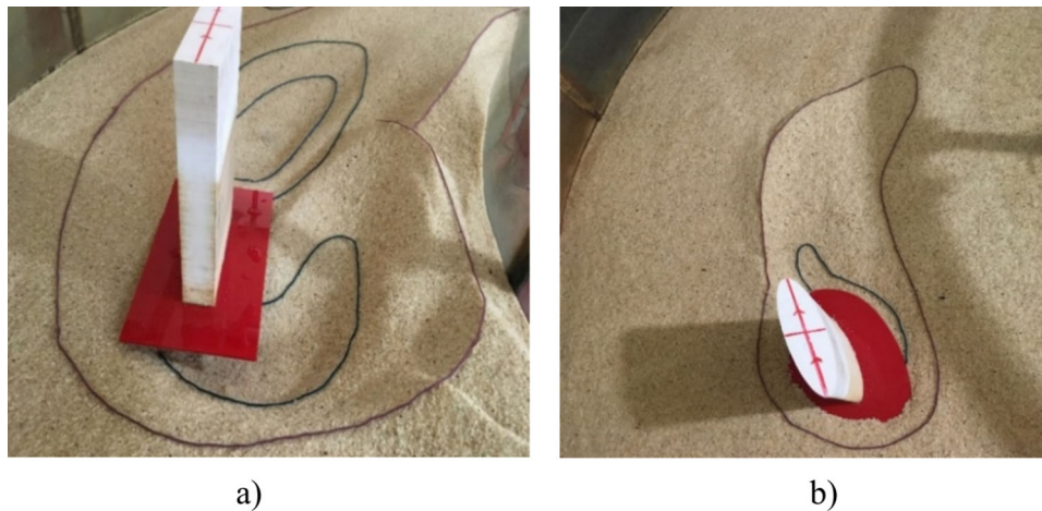
Fig. 3 Hole created around a the rectangular pier installed at 90^\circ , and b the elliptical pier installed at 120^\circ
