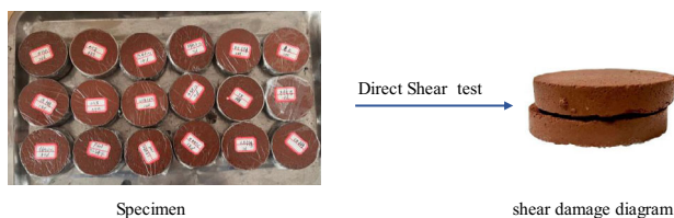
Fig. 6 Direct shearing specimen diagram
