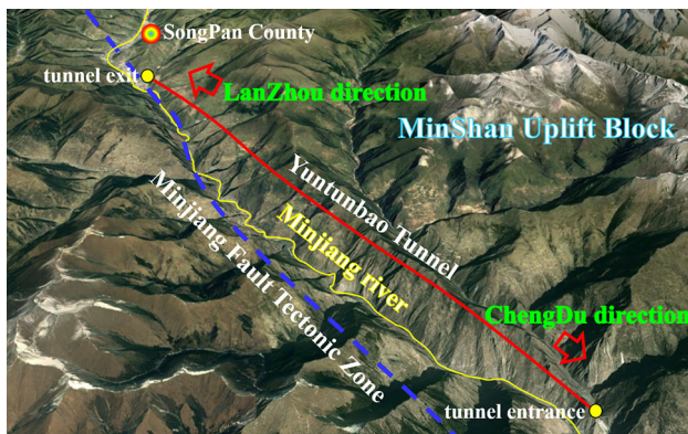
Fig. 2 Schematic diagram of the relationship between Minjiang fault zone and tunnel line
