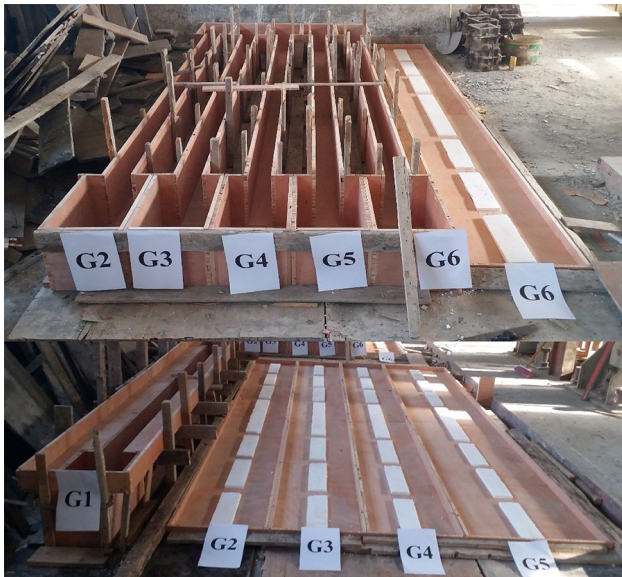
Fig. 7 Preparation of formwork for tested specimens
