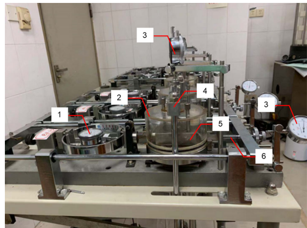
Fig. 5 Improved triplex rheology direct shear creep apparatus: 1: indicators of shearing force; 2: moisturizing seal box; 3: indicators of normal and shear displacements; 4: normal load; 5: shear box; 6: shear load
