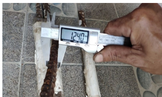
(a) Measuring diameter of rebar after corrosion
