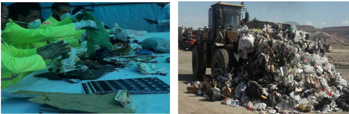
Fig. 3 The process of mixing, separating and analyzing the MSW sample
