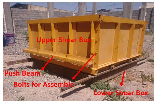
Fig. 5 The device's main parts
