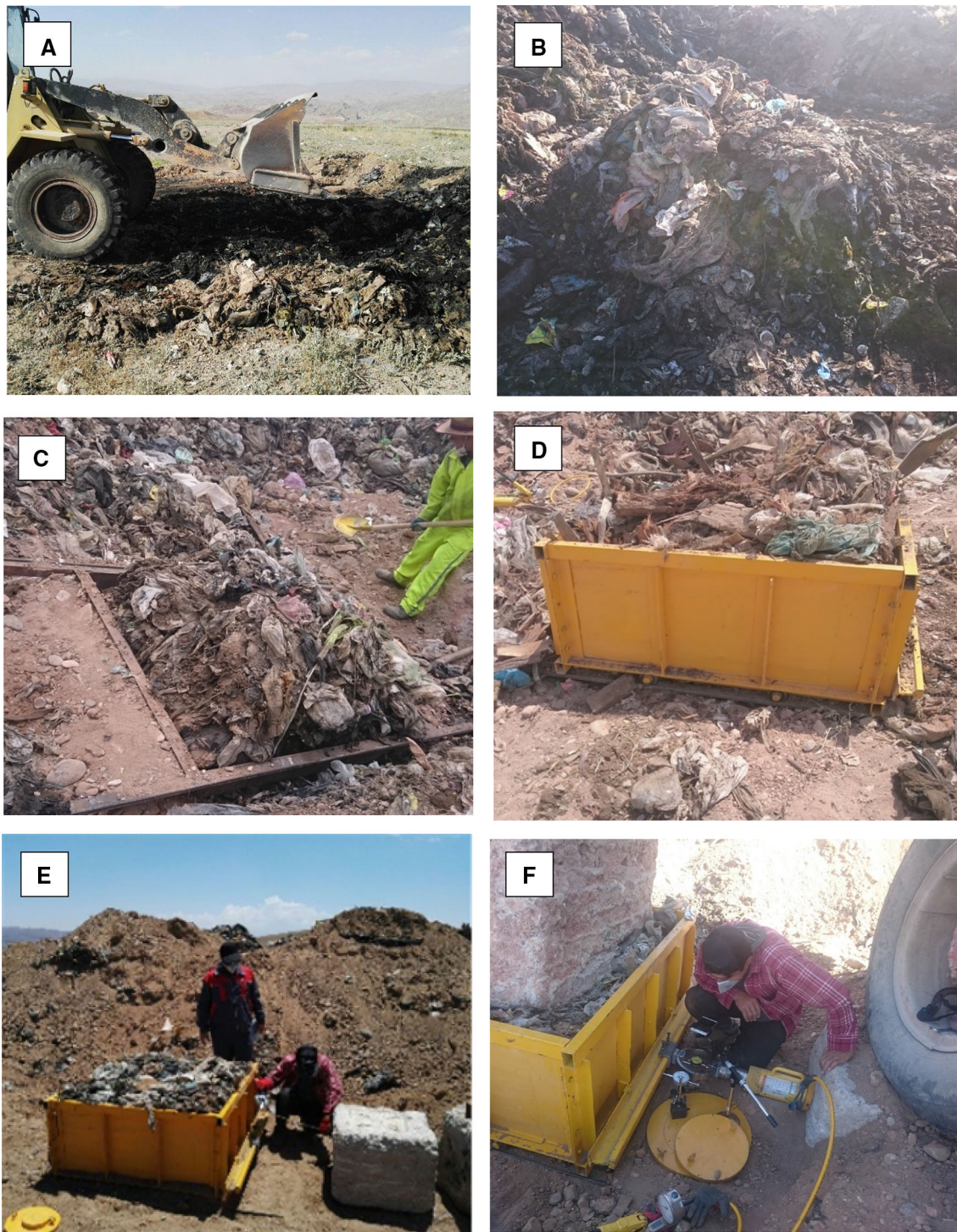
Fig. 8 Large-scale in situ direct shear experiment steps (a removing the coating, b preparing a sample with approximate dimensions of 122 \times 122 cm, c placing the lowest part of the box, d placing the upper box around the sample, e placing support, f fitting the box to a jack and displacement gauge and applying normal stress)
