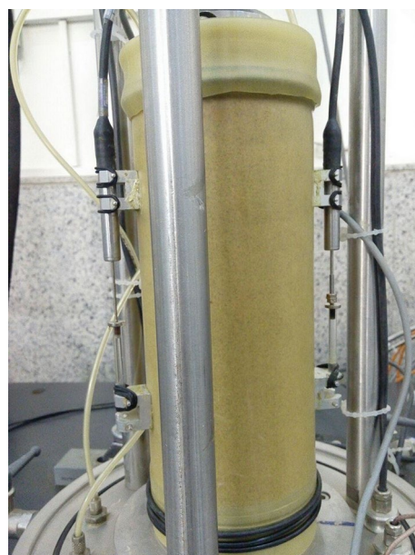
Fig. 4 Prepared specimen along with two LVDTs
