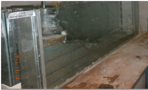
Fig. 12 Slope failed under a pressure of 7.8 kPa (Model 2)
