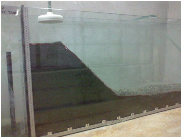
Fig. 5 Slope made of sand with a slope angle of 45°
