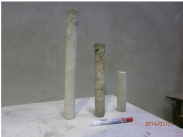
Fig. 3 Concrete piles used at different locations along the slope
