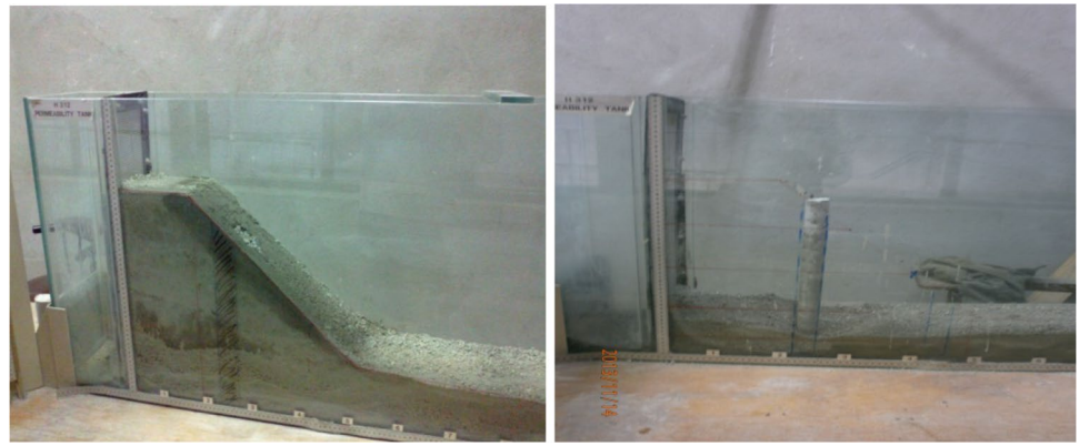
Fig. 11 A concrete pile with a diameter of 3.6 cm installed at x/r=0.75
