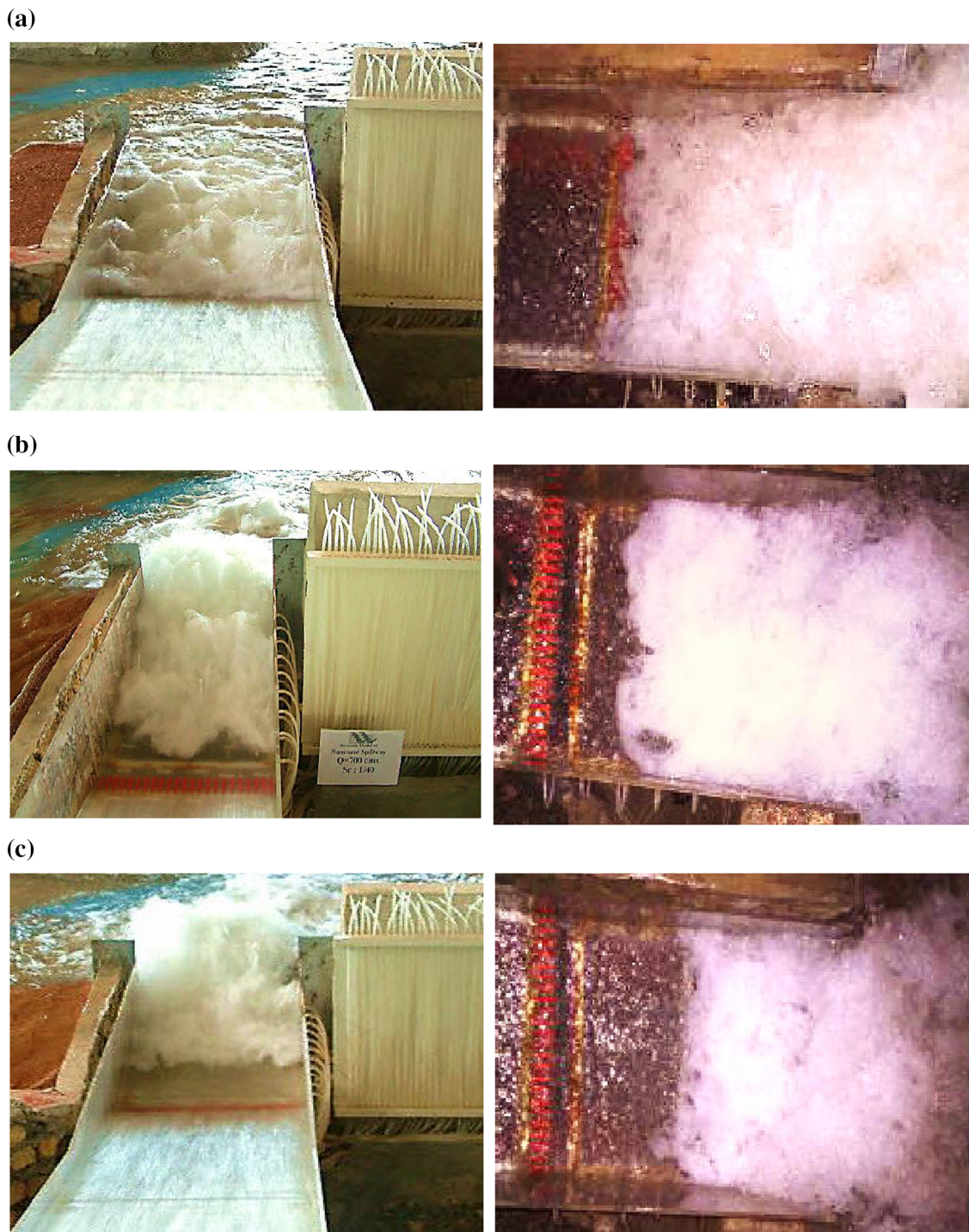
Fig. 2 Formation of hydraulic jump at different discharges [24, 26]
