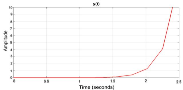
Fig. 2 Step response of the open-loop system
