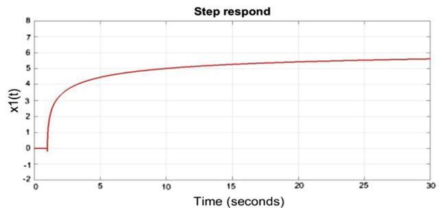
Fig. 3 Step response of the closed-loop system
