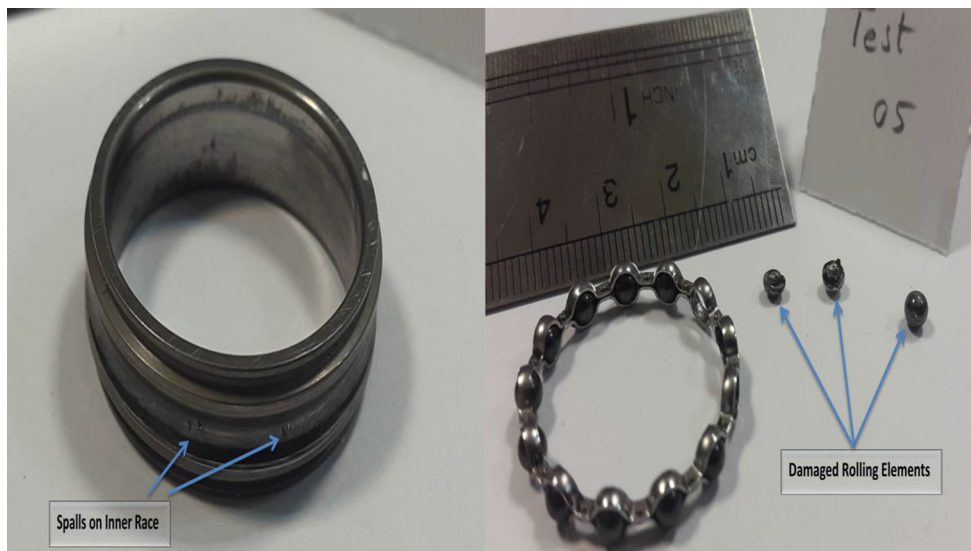
Fig. 6 Inner race and rolling elements of the damaged bearing in test no. 5
