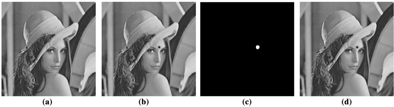
Fig. 6 a The watermarked Lena, b tampered Lena, c actual tampered areas, and d located tampered areas
