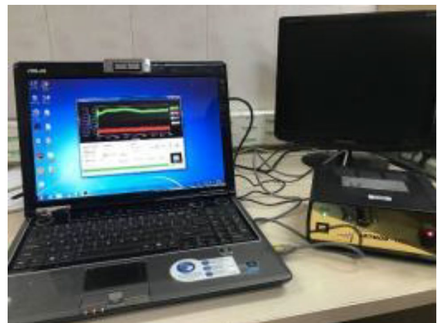
Fig. 4 Measurement of the natural frequency of aluminum sheet using modal analysis
