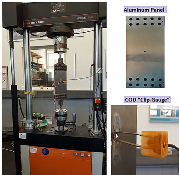
Fig. 5 AA7075-T6 Aluminium Panel fitted with COD “Clip-Gauge”
