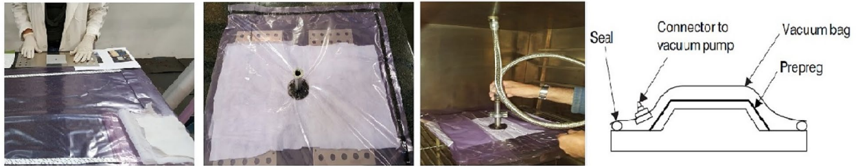
Fig. 3 Detail of vacuum bag lay-up
