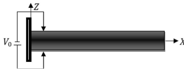
Fig. 1 Schematic view of a flexoelectric nanoactuator
