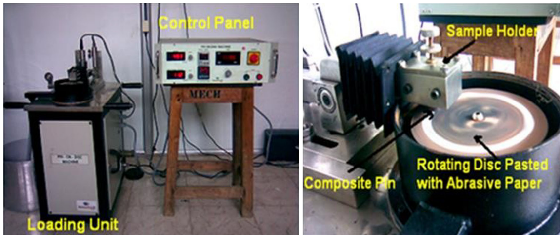
Fig. 3 Experimental set-up of abrasive wear test on pin-on-disc wear tester
