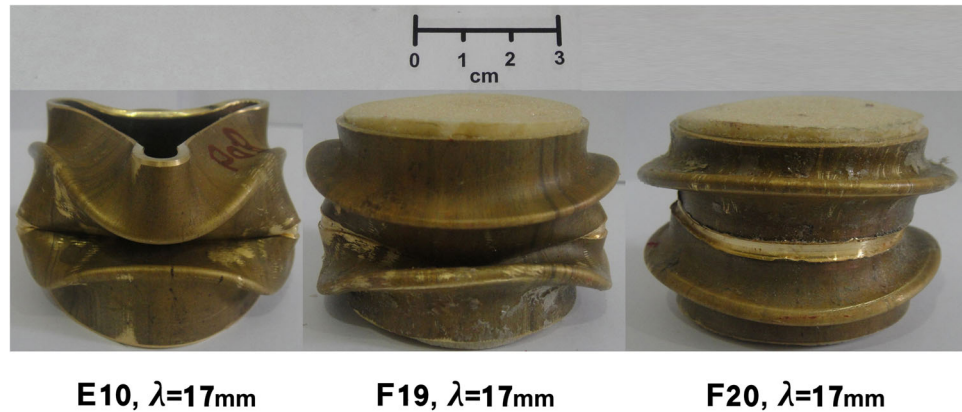
Fig. 17 Deformation modes of the foam-filled grooved specimen F19 and F20 and empty grooved specimen E10 with the same grooves distance
