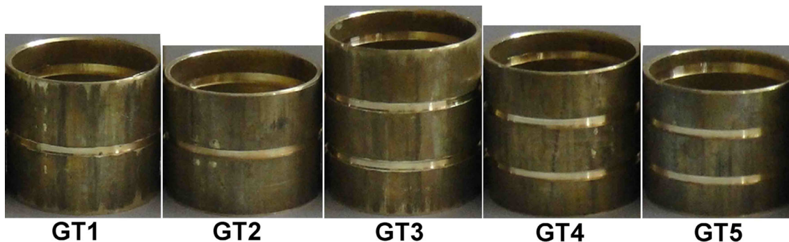
Fig. 5 Empty circular grooved tubes before the tests
