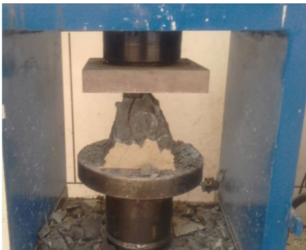
Fig. 4 Compressive strength test device
