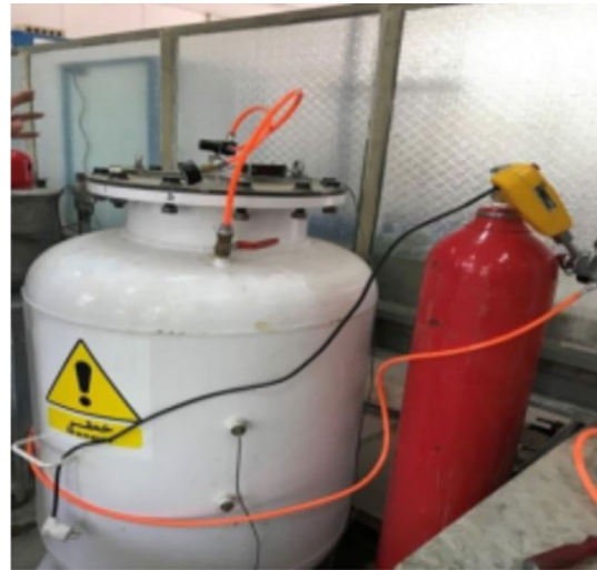
Fig. 3 Carbonation depth measurement test device
