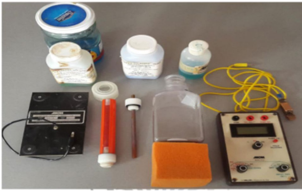
Fig. 2 Half-cell potential measuring instruments
