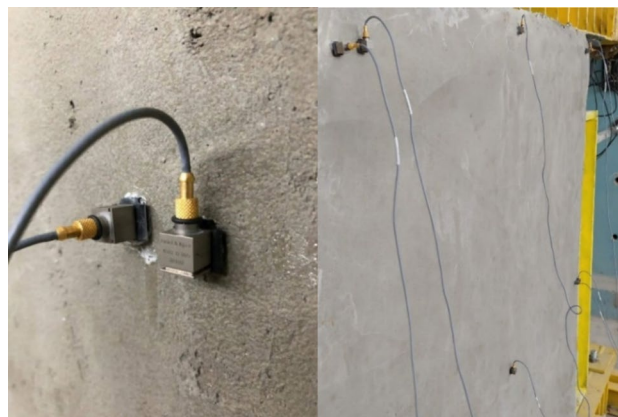
Fig. 14 The location of the mounted point of accelerometers on SMW
