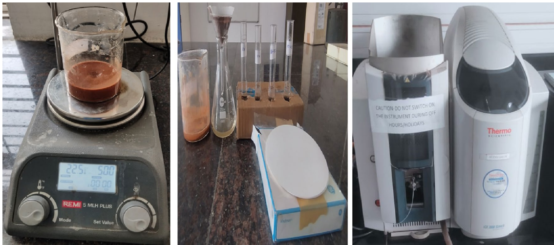
Fig. 3 TCLP test set up with specimens
