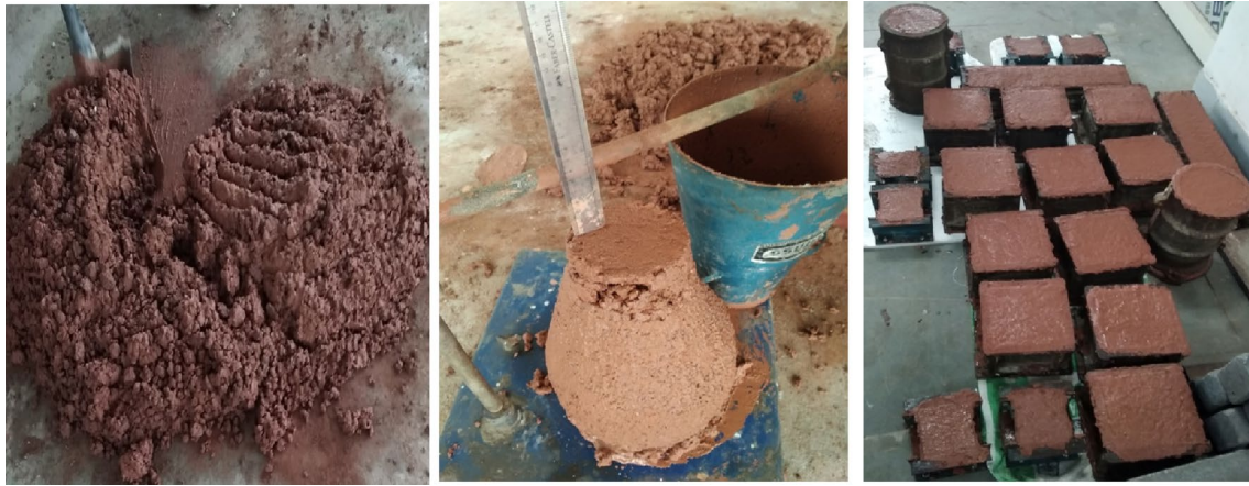
Fig. 1 Photograph of experimental work during mixing and casting of specimens
