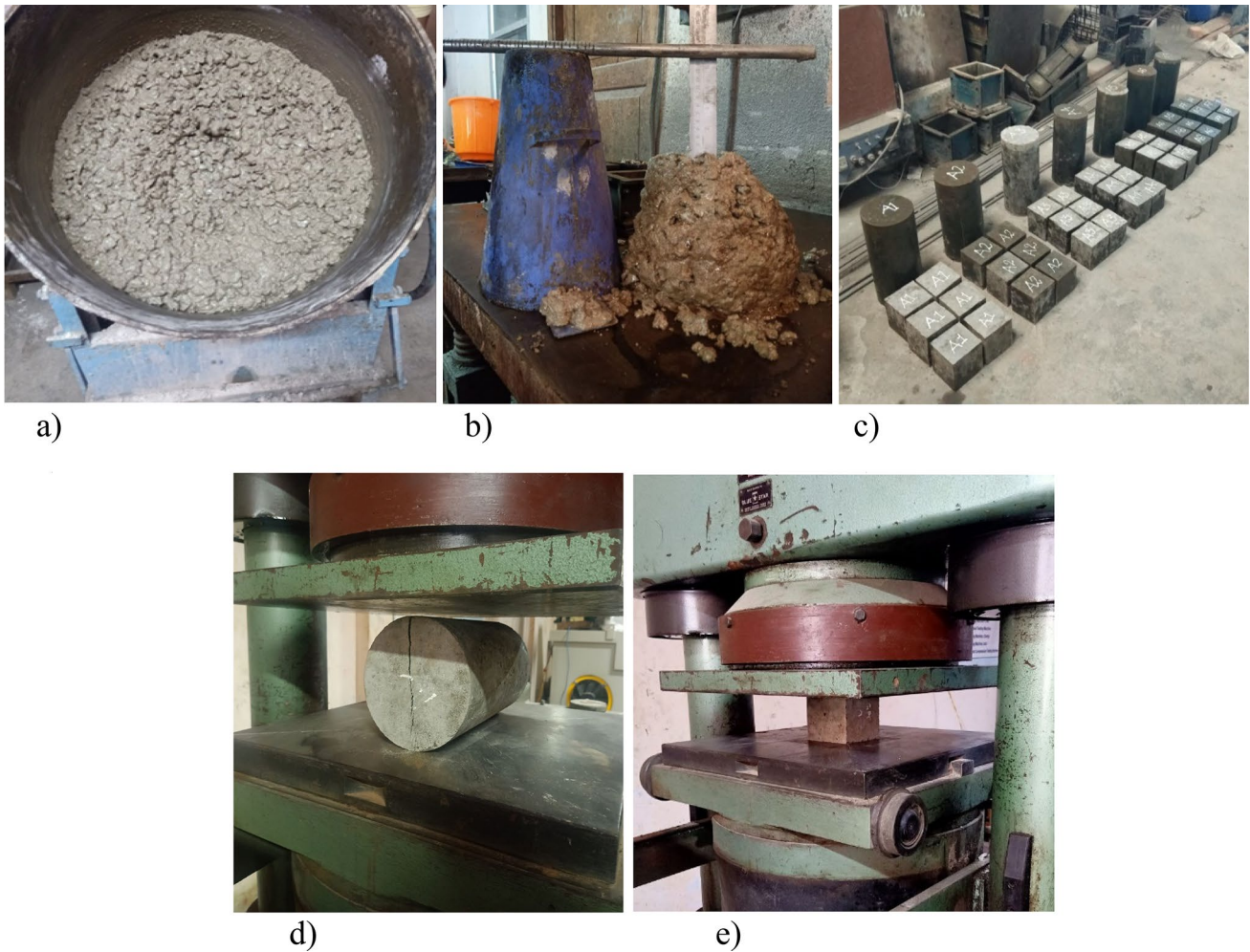
Fig. 4 a GPC mix in pan mixer b slump test c Cast specimens subjected to ambient curing e Split tensile strength test f Compressive strength test
