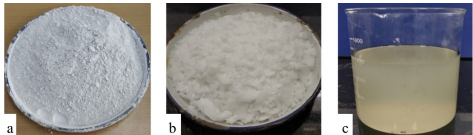
Fig. 1 Images of a GGBS, b sodium hydroxide pellets, and c sodium silicate liquid
