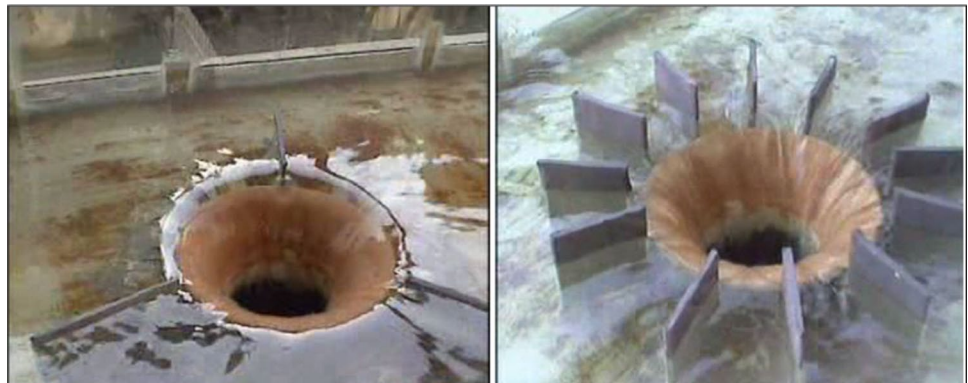
Fig. 12 A view of the shaft spillway’s physical model with different VB numbers in the laboratory (Akbari et al. 2015)
