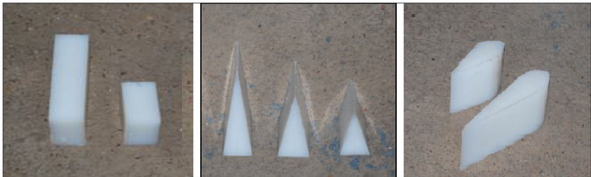
Fig. 11 Different sizes of rectangular, triangular, and baleen body anti-vortex blades (Nohani and Emamghais 2015)
