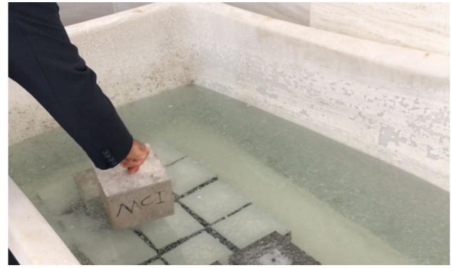
Fig. 1 Curing concrete specimens
