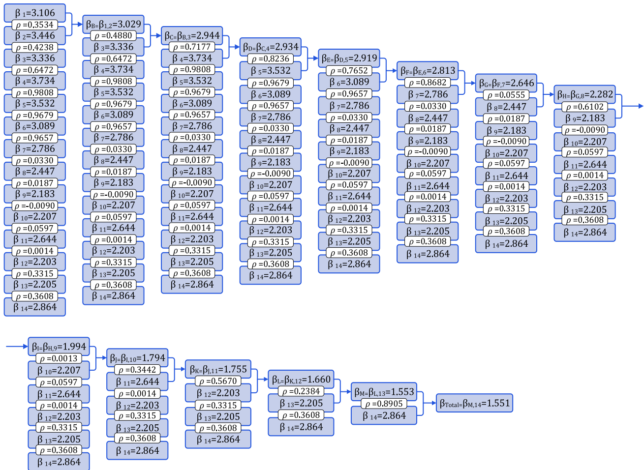
Fig. 20 Determination stages of the system reliability index for the global safety factor
