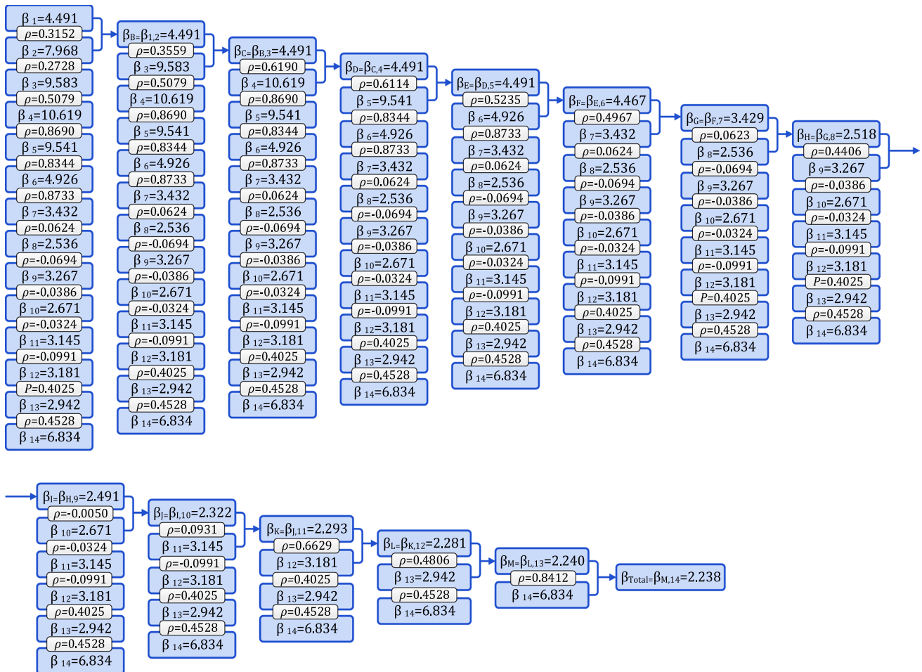
Fig. 21 Determination stages of the system reliability index for the maximum horizontal displacement safety factor
