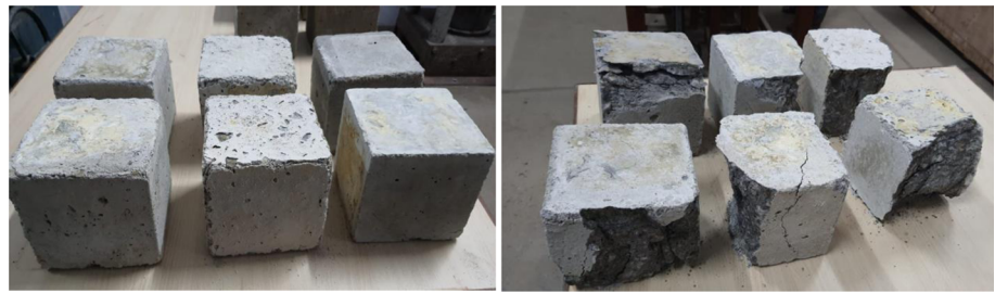
(a) Samples exposed for 6months immersed in 5% of sulphuric acid
