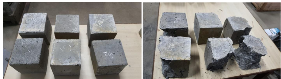
(c) Samples exposed for 6months immersed in 5% of Sodium chloride
