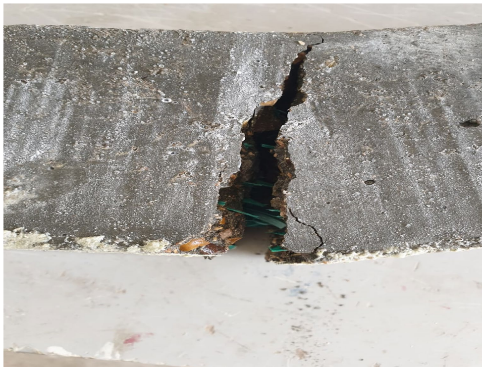
Fig. 19 The sample after the flexural test
