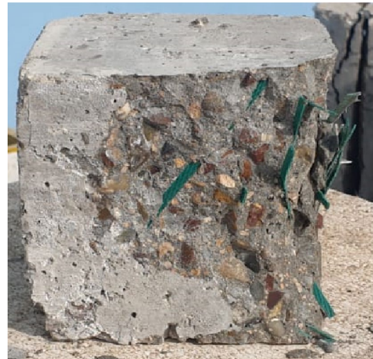
Fig. 17 The sample after the compressive test
