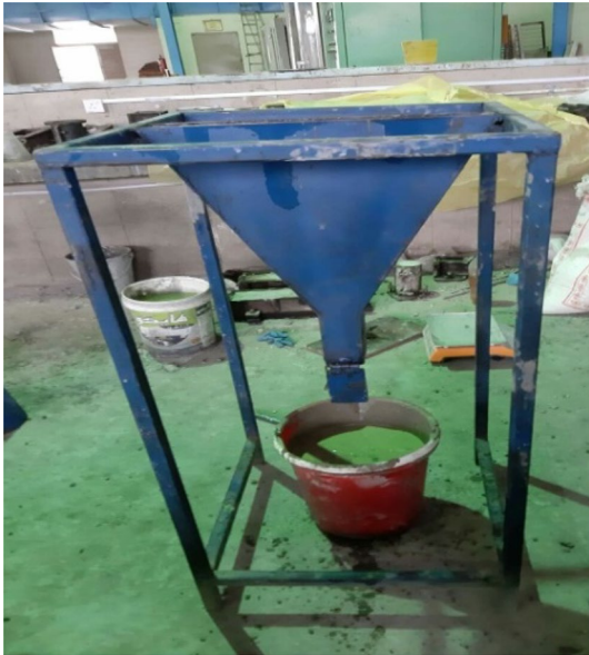
Fig. 7 V-funnel test process
