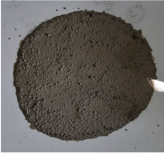
Fig. 6 Slump flow test
