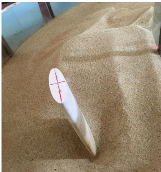
Fig. 12 The scour hole created around a The round pier place at the angle of 60-degree b The elliptical pier place at the angle of 120-degree
