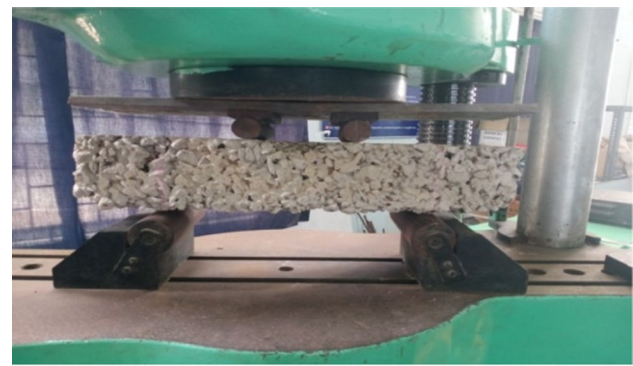
(a) Flexural test Setup Two-point Load condition
