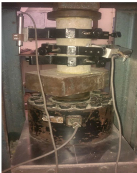
Fig. 4 Cylinders tested to compression
