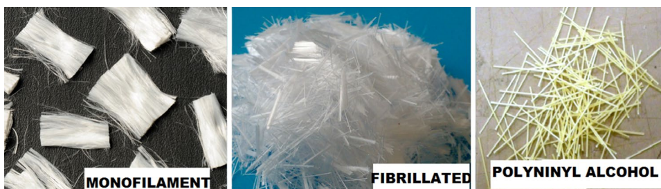
Fig. 1 Polypropylene (monofilament and fibrillated types) and polyvinyl alcohol fibres used
