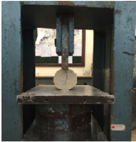
Fig. 7 Cylinder tested for a split tension
