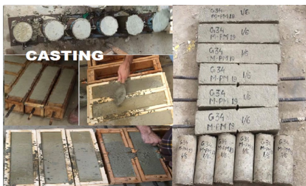
Fig. 3 Specimen casting detail
