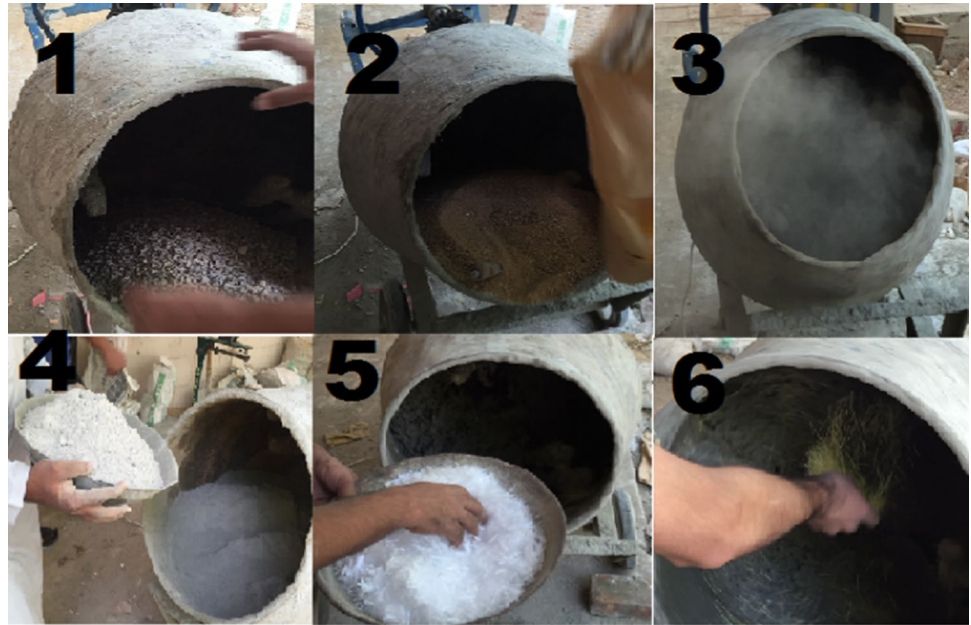
Fig. 2 Hybrid SCC-FRC mixing sequence
