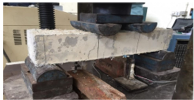
Fig. 9 Flexure test set-up
