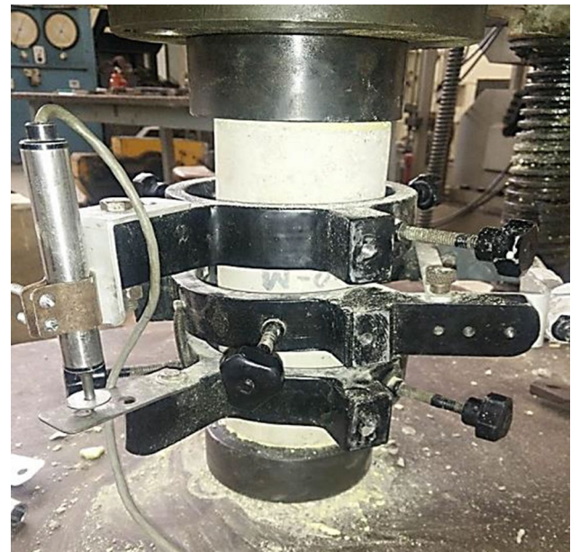
Fig. 2 Setup of compressive strength test
