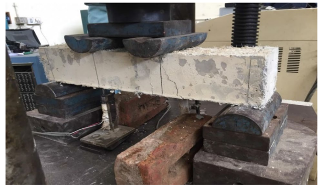
Fig. 10 Flexural test arrangement
