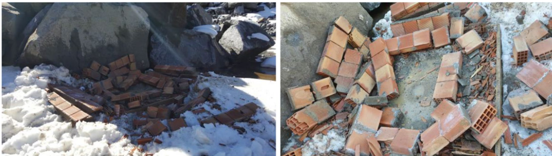
Fig. 6 The collapsed masonry walls after blasting test performed with 290 g TNT explosive
