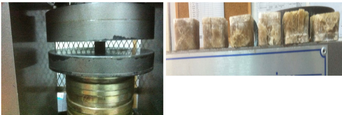
Fig. 3 Compressive stress test at 10% relative deformation
