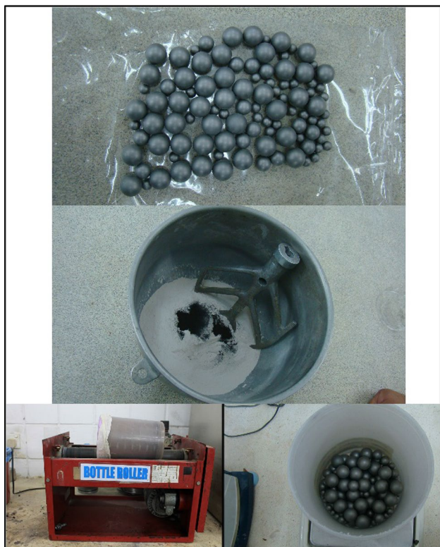
Fig. 4 Horizontal ball mill mixing of nano-copper oxide with kaolin-ite (Firoozi et al. 2019)
