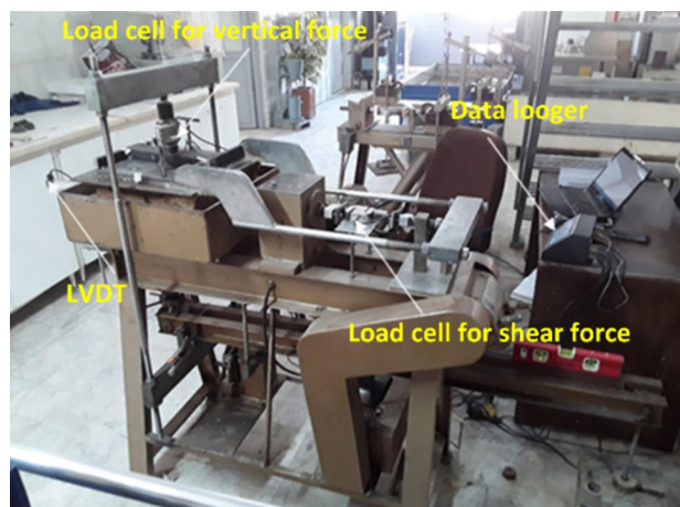
Fig. 3 Direct shear device and installed equipment
