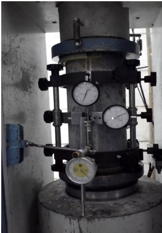
Fig. 5 Instrumentations for the concrete cylinder in the compression test
