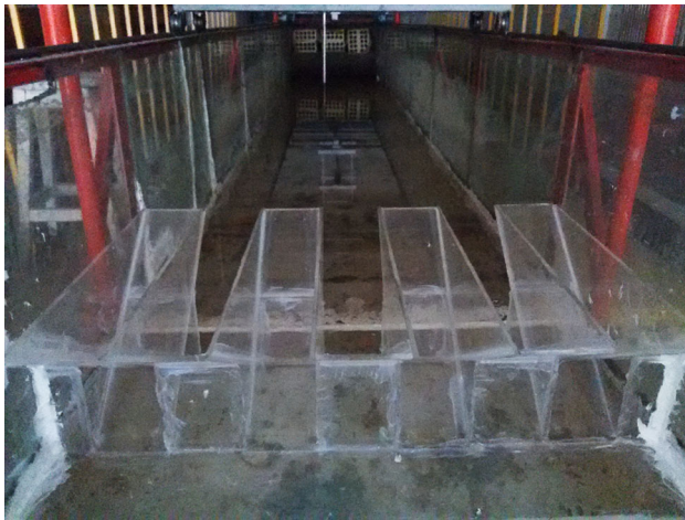
Fig. 2 Overview of weir test setup
