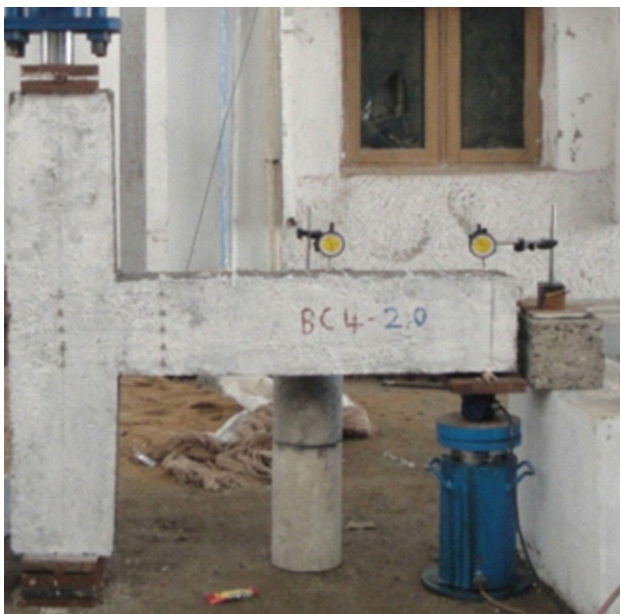
Fig. 6 Beam-column joint specimen testing setup in loading frame
