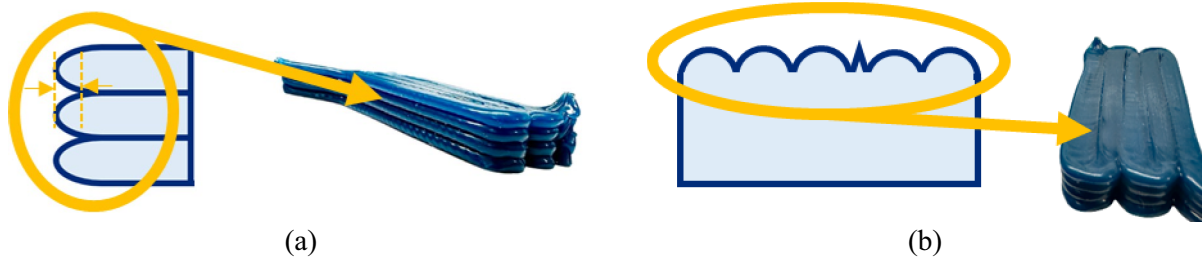
Fig. 7 Response variables selected for the DoE a stair-stepping depth and b valleys and ridges
