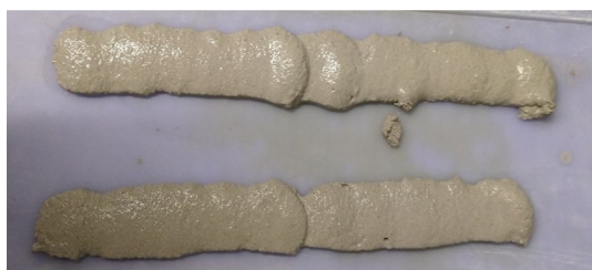
Fig. 10 Printed mixes using auger screw system using mix No. 20
