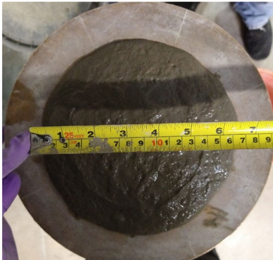
Fig. 11 Result of flow table test, conforming to ASTM C1437 [52]
